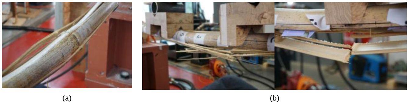
Gambar 34(a) Tensile perpendicular to the fibers dan (b) Failure due to tensile stresses in fiber direction at the nodes oleh Fritz et al (2025)
