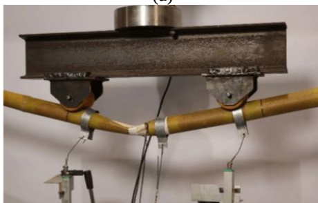
Gambar 32 (a) Local crushing , (b) Longitudinal shear cracking along the neutral axis followed by buckling , (c) Local buckling , (d) Splitting followed by rupture at the tension layer , oleh Seixas et al (2024)
