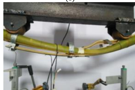
Gambar 32 (a) Local crushing , (b) Longitudinal shear cracking along the neutral axis followed by buckling , (c) Local buckling , (d) Splitting followed by rupture at the tension layer , oleh Seixas et al (2024)
