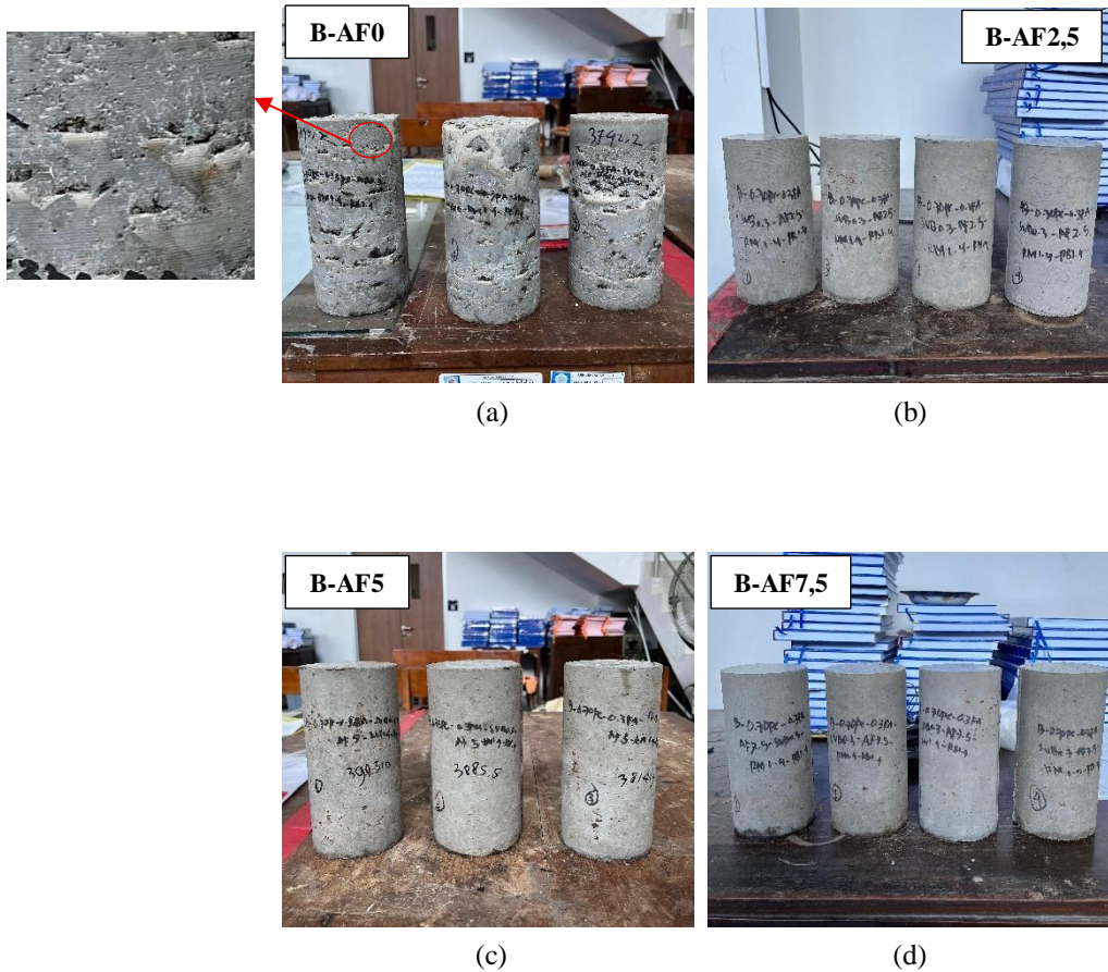
Figure 3. The condition of the concrete after 24 hours of curing (a) concrete without alkali activator; (b) concrete with 2.5% alkali activator; (c) concrete with 5% alkali activator; (d) concrete with 7.5% alkali activator.
