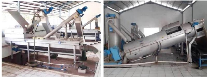
Gambar 4. Unit pengolahan mekanis di IPLT Duri Kosambi dan IPLT Sumur Batu
